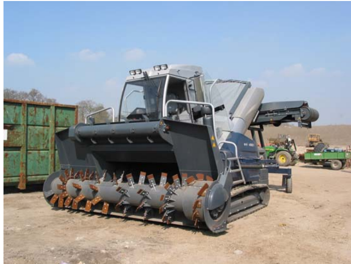
Plate2: Windrow turner (Sandberger UNI 4001) used in enclosed composting hall
